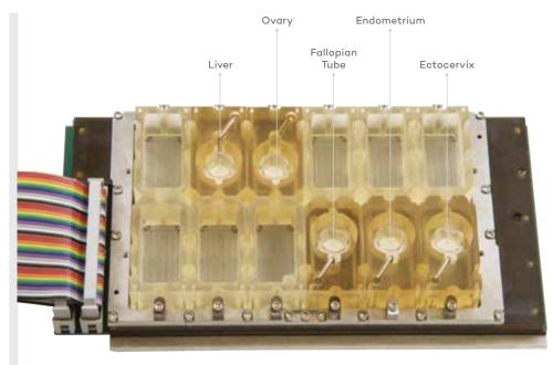
EVATAR is a female reproductive tract that fits in the palm of one's hand. Each divided compartment within the cube contains a 3-D model of a different part of the reproductive tract, a personalized model of the reproductive system to test new drugs for safety and effectiveness.
