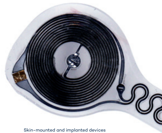
Skin-mounted and implanted devices monitor body temperature, oxygen levels, respiration, muscle tone, physical activity, and the heart’s electrical activity.
